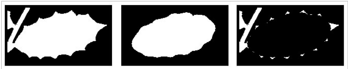
Figure 3.9: Left to Right - Original Binary Image, Core Leaf Body, Possible Regions for Removal
