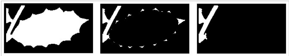
Figure 3.10: Left to Right - Original Binary Image, Possible Regions to Remove, Regions Selected for Removal
